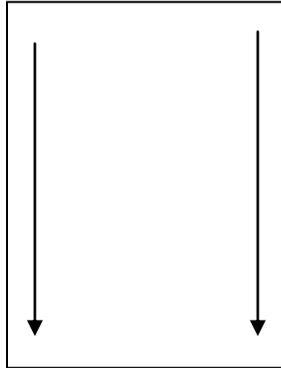
7. Second Wipe Pass (top-to-bottom). Repeat the above procedure using the same wipe and S-like motion but at a 90° angle to the first. Attempt to remove all visible dust or paint chips. Fold contaminated side inward again and insert wipe into centrifuge tube (one wipe per centrifuge tube.)
